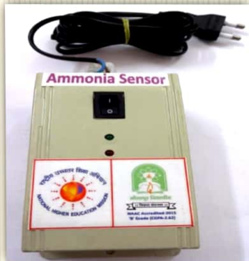
Developed Ammonia Gas Sensor (Device)- AC operated
